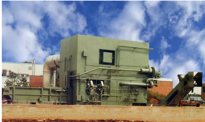
Pharmaceutical Waste Treatment System with Heat Recovery and Automatic Ash Removal
